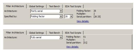
When you click on the **View details** link, the coder displays an HTML report in a separate window. The report displays an exhaustive table of folding factor, multiplier, and serial partition settings for the current filter. You can use the table to help you choose optimal settings for your design.
